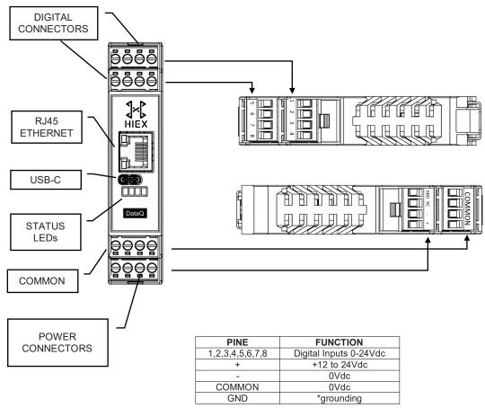
\*must not be connected to the 0V of the power supply.
